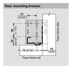
**NOTE:** For use in frame applications, minimum three screws per bracket
