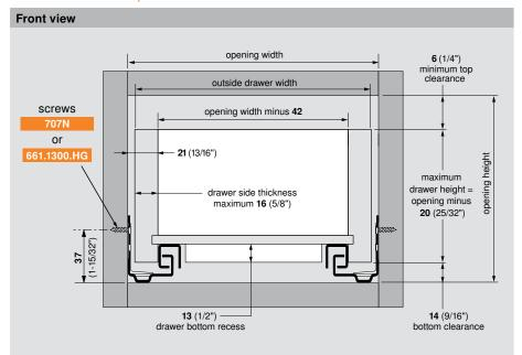
NOTE: Because material thickness may vary, the inside drawer width **must** equal opening width minus **42** for TANDEM to align and function optimally.
