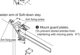
6 Guard plate(H)  $\langle$ %<sup>4</sup> If the gaurd plates are not enough to avoid interference install a middle plate.
