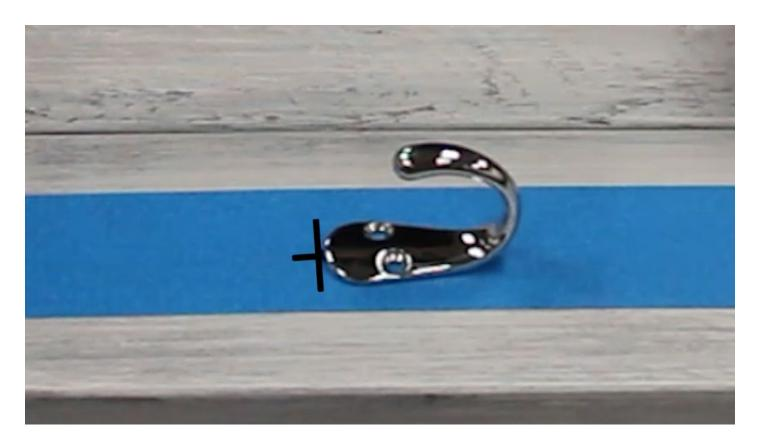
**Step 11:** Using a pen or a pencil, mark the placement of the hooks on the board. Then, place the hooks on the board and mark the screw holes in the hooks onto the tape. Remove the hooks from the project.
