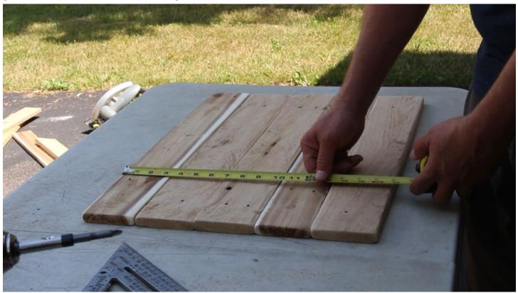
**Step 6:** We'll cut (2) braces to hold everything together. Using another piece of the pallet wood or even leftover wood scraps from your previous cuts, measure and cut (2) 16-1/2" long braces. Our pieces were about 16-½" by 3-½". Test the placement of the braces across all 5 boards to be sure everything lines up and the braces do not hang over the edges of the boards.
