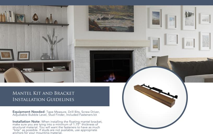
**Step 1**: Choose a mounting position on the wall and find stud locations within the length of the bracket. Position the bracket using a level and mark at the slots which align with the stud locations. You do not need to mark at every slot provided on the bracket, just the ones that align with the stud locations. Drill pilot holes, using a 1/8" or 3/16" drill bit.
