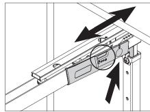
Carefully pull down locking mechanism and adjust to weight of pay load
