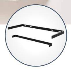
black finish and includes screws to attach the inner gusset rib. Four slots are provided for adjusting the placement as needed. Slots are sixteen inches on center. Arms extend from both ends of the bracket for insertion into the floating shelf box.
