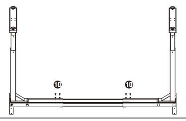
Η. Double-check that the base is centered on the underside of the desktop and is located where you want it. Also, double-check that the included wood screws are not too long for your desktop and won't puncture the surface when screwed all the way in.
