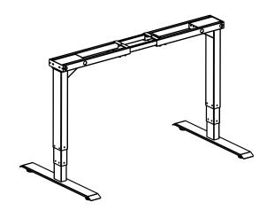
D. Put the 2 side brackets #5 on two sides of the frame, and then put 2pc Flat head screw #14 on the side brackets and then tighten.
