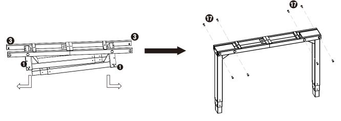
B. Put the two feet on the legs, and then attach each feet with 4 Machine screw #10, and then make sure tighten bolts in a cross pattern.Next put 2pcs leveling studs # 8 on each leg, and tighten them
