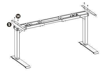
Ε. The Crossbar Center Rails (Part #4) are optional. They provide more stability but if not needed they can be skipped during installation or removed later. Slide Crossbar Center Rails (Part #4) back into Crossbar Ends (Part #3). Ensure the slots of the Crossbar Center Rails are facing inward.
