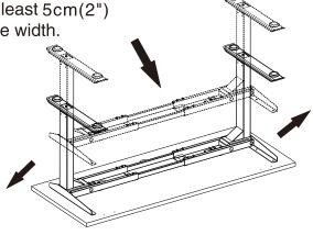
G. Secure the Center Rails at both ends using qty 8 Machine Screw (Part #10), qty 4 per side.
