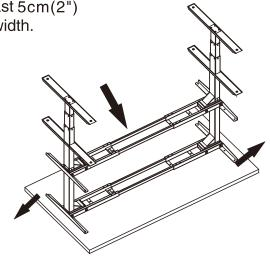
G. Secure the Center Rails at both ends using qty 8 Machine Screw (Part #10), qty 4 per side.
