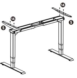
E. The Crossbar Center Rails (Part #4) are optional. They provide more stability but if not needed they can be skipped during installation or removed later. Slide Crossbar
