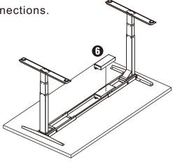
J. IN THIS FOLLOWING STEP, DO NOT OVERTIGHTEN SCREWS. OVER TIGHTENING COULD CAUSE THE PLASTIC ON THE COMPONENTS TO BREAK.
