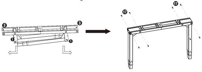
B. Put the two feet on the legs, and then attach each feet with 4 Machine screw #10, and then make sure tighten bolts in a cross pattern. Next put 2pcs leveling studs # 8 on each leg, and tighten them
