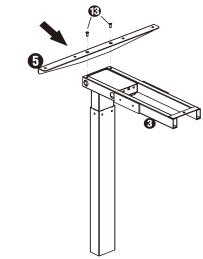
Assemble the Crossbar End(part#3), 2pcs as the picture and SideBracket(Part#5) to the Center Leg(Part#1) with qty 6 M6x12 Machine Screws (Part#10). Install M6x8 flush head screws (part 13) as shown.
