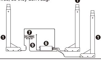
M. Turn the assembled desk right-side-up. With two people, grab the desk by the base (not the desktop) and turn the desk right-side up. Adjust the Leveling Studs on the Feet (Part #9) as needed.
