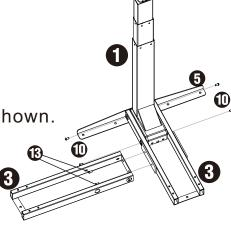
Once all of these screws have been started, you can now tighten the qty D. 6 Flat Head Screws (Part #13) from Step C and the qty12 Machine Screws (Part #10) described in Step B (18 screws in total).
