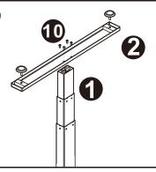
Your desktop may or may not be pre-drilled. Please check both sides of the desktop before G. placing the desk base on it for pre-drilling! Carefully place the upside down desk base on the underside of the desktop.
