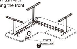
L. Connect the Wires as per the diagram below. Use the adhesive-backed Cable Clips (Part #12) to secure the Connecting Wires, so they don't sag.
