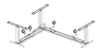
I. Double-check that the base is centered on the underside of the desktop and is located where you want it. Also, double-check that the included wood screws are not too long for your desktop and won't puncture the surface when screwed all the way in.
