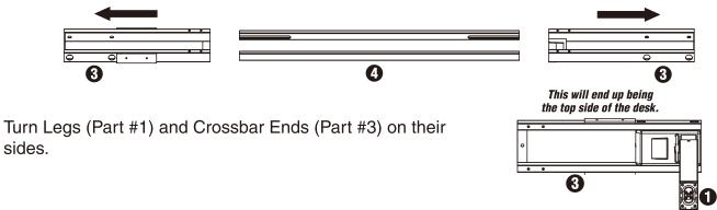
Line up the holes on each Leg (Part #1) with the holes on each Crossbar End (Part #3).
