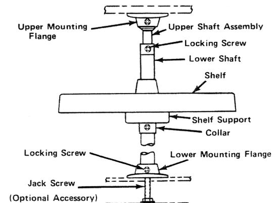
\* Mounting flanges are tapped for jack screw accessory. If used, drill 1" diameter hole through bottom floor only.
