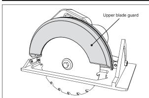
ATTENTION The Accu-Cut™ is designed for use with portable circular saws that have a metal upper blade guard. When paired with the Accu-Cut, a saw with a plastic upper blade guard may allow deflection between the blade and the base plate resulting in poor cut quality. Do not use a saw with a plastic upper blade guard with the Accu-Cut.
