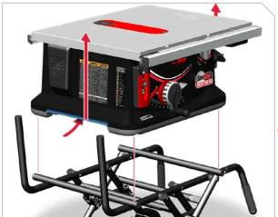
Use the hand grips to lift saw straight up and off cart. To re-attach saw, reverse steps.
