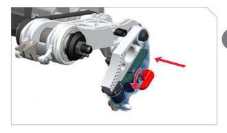
Slide new brake onto both pins. Insert key and rotate 1/4 turn counter-clockwise to lock in place. Reinstall riving knife/blade guard and table insert.
