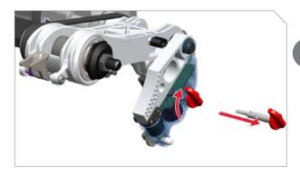
Turn brake key 1/4 turn clockwise and pull out.
