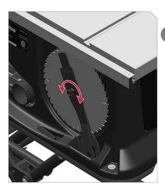
Switch power off and unplug power cord. Remove table insert and riving knife/blade guard. Release wrenches by turning knob 1/2 turn.
