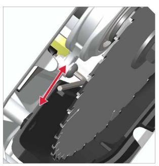
Locate adjustment bolt, which is down and left of blade, inside table insert opening. Use 4 mm hex key wrench to rotate bolt clockwise to move blade right, and counterclockwise to move blade left. Once adjusted, tighten arbor nut. Return to step 2 and make further adjustments as necessary.
