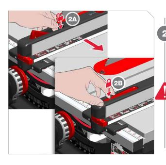
To move the fence, push lever down to unlock the fence (2A), and then slide fence until the indicator line reads desired cut width. Push down on the opposite end of the lever (2B) to lock the fence in place.
