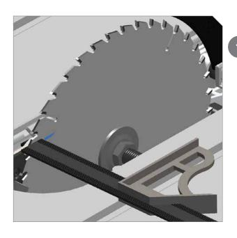
Remove table insert and raise blade. Set combination square parallel with right miter slot. Extend ruler until it touches space between two teeth at front of blade. Mark that point on blade. Note ruler measurement.
