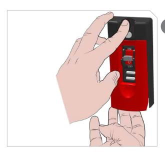
While pressing bypass switch, pull paddle out to spin blade. Keep pressing switch until red light flashes once, then release switch.
