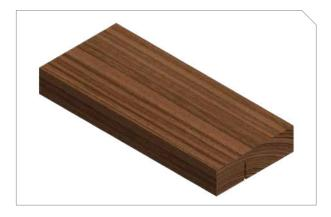
A non-through cut does not extend through the entire thickness of the workpiece. In this case you cannot use the blade guard and splitter but must use the riving knife instead.
