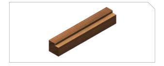
A rabbet cut is used to create a rectangular notch along the edge of a workpiece.
