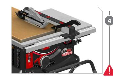
Make sure workpiece is not touching blade when starting motor.
