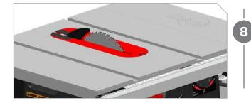
Stop motor and turn saw off. Remove wood and clamps. Remove table insert and install riving knife or blade guard (see page 30). Reinstall insert.
