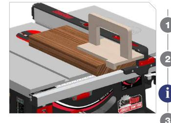
Adjust blade elevation to desired cut depth. Position fence at desired width and lock in place.
