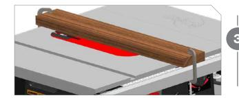
Clamp a thick piece of wood across right side of table insert to securely hold table insert to table.
