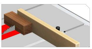
As needed, flip workpiece over and make another series of cuts, offset from first set, using same method.
