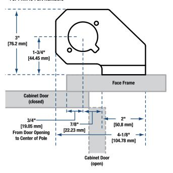
NOTE: For frameless cabinet applications, move bracket 1-1/4" [31.75 mm] toward cabinet opening. NOTE: For frameless cabinet applications, move bracket 1-1/4" [31.75 mm] toward cabinet opening.
