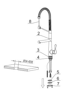
1. Remove the mounting hardware(7), metal washer(6) and rubber washer B (5) from the main body (2).
