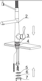
2. Insert the main body into the hole with base(3) and rubber washer A(4) . Refix the rubber washer B(5), metal washer(6), mounting hardware(7) from the bottom.
