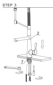
After adjusting the direction of the main body(2), tighten the mounting hardware (7) with hands and tighten the screws with a Philips screwdriver.
